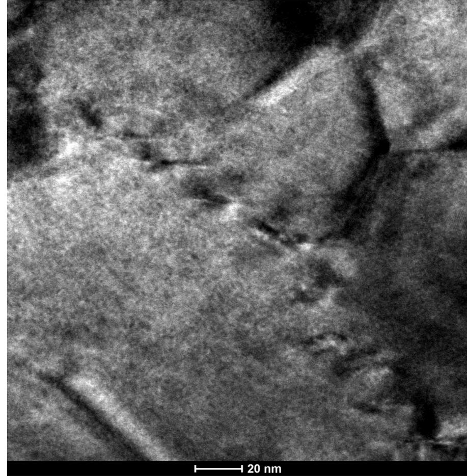
Precipitates are formed in a sequence due to formation of each one in the strain field of the other one which after deformation can form grain boundary
