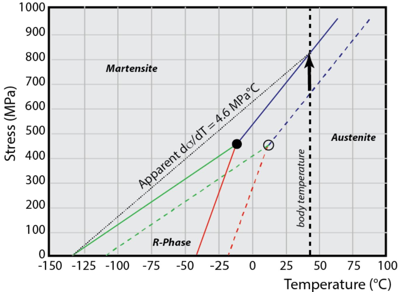
$$(d\sigma/dT)_{\text{apparent}} = [(T - T_o)(d\sigma/dT)_{A-M} + (T_o - M_p)(d\sigma/dT)_{R-M}] / (T - M_p)$$
