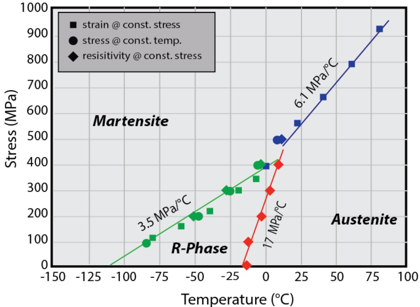
If the slopes are “crystallographically fixed,” extrapolating to the zero-stress transformation temperatures defines the entire diagram
