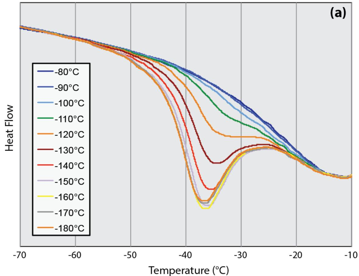
Integrating the reversion peaks allow one to identify martensite formation temperatures
