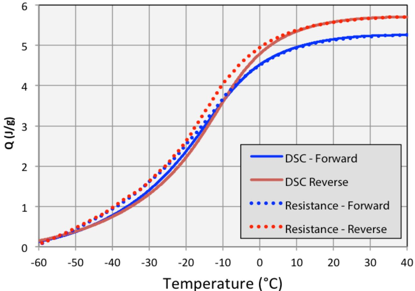
Calculating  $d\sigma/dT$  from DSC fails even in the A-R case
