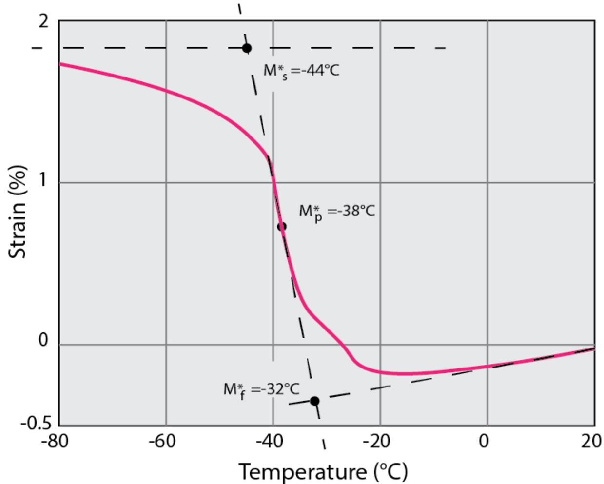
\* Deformed 2% in tension at  $-100^\circ\text{C}$ , released, and warmed at  $5^\circ\text{C}/\text{min}$ .
