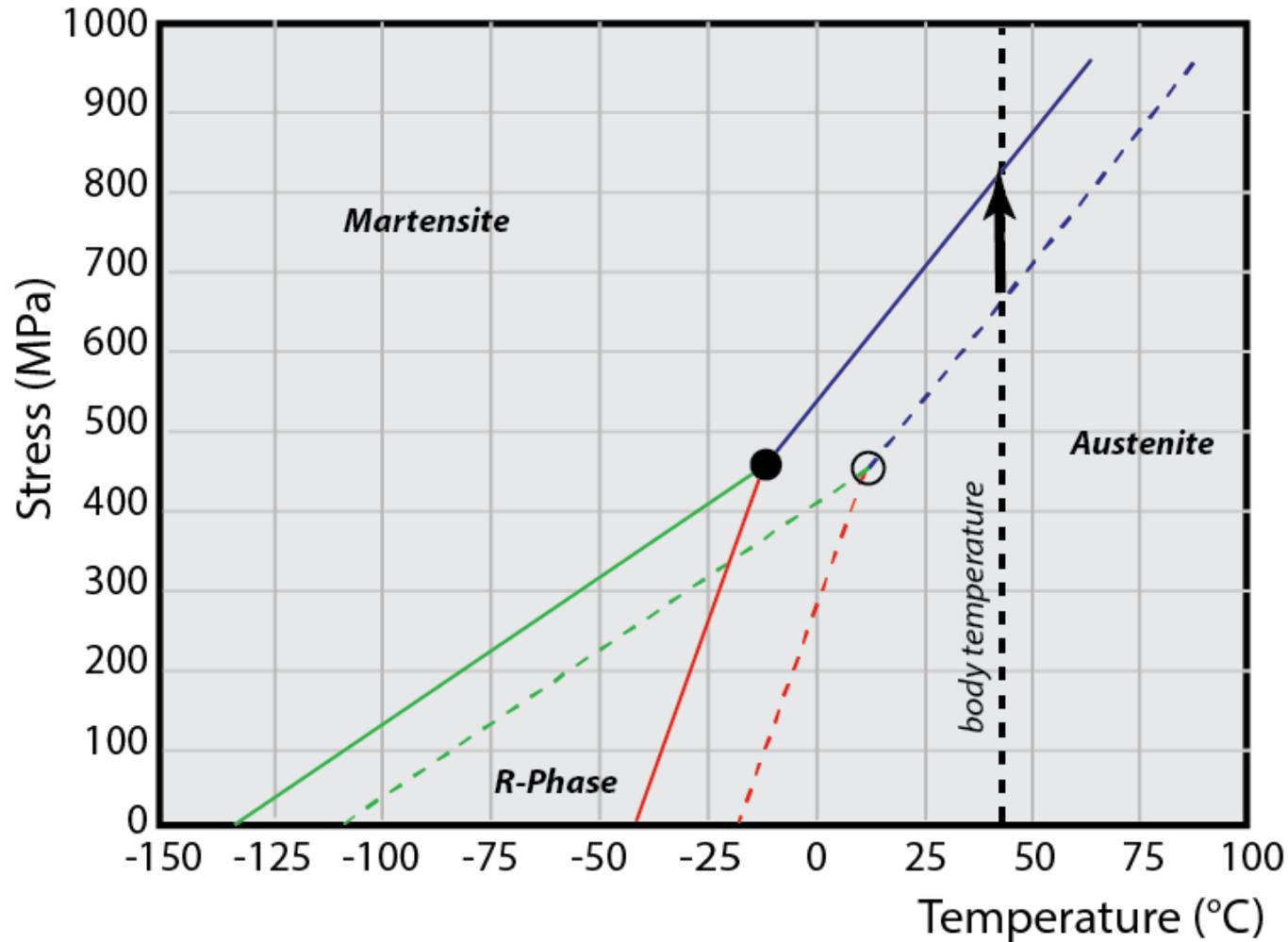
Apparent  $d\sigma/dT$  is an average weighted from the triple point
