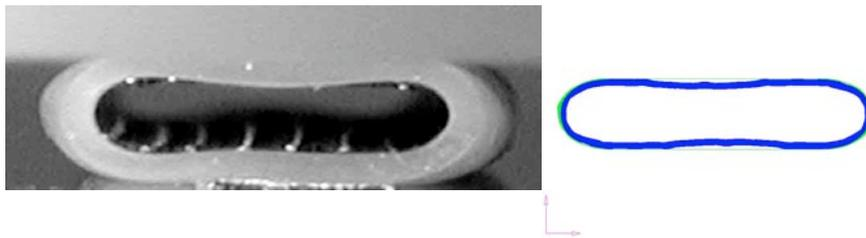
*Figure 9. Comparison of deformed stent shape from experiment (left) and FEA (right)*
