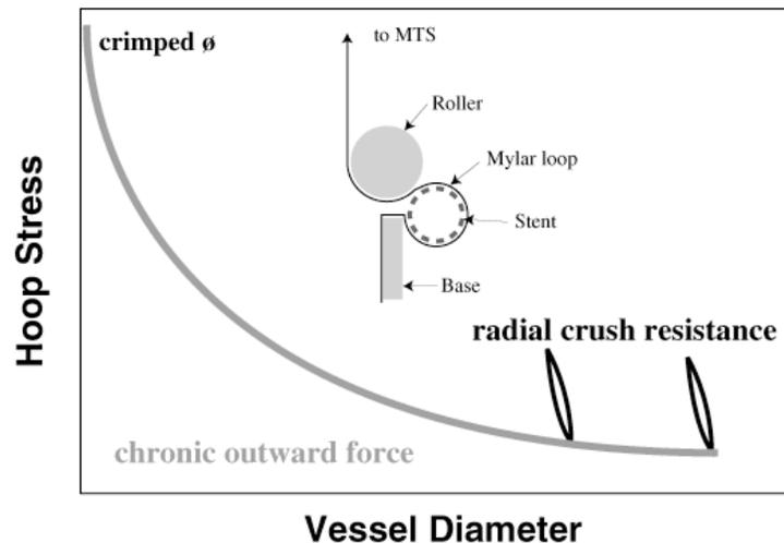
Figure 3. Schematic radial force test set up
