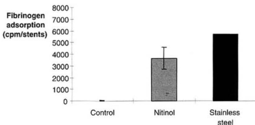
Figure 3  $^{125}\text{I}$ -fibrinogen adsorption on Nitinol stents, SS stents, and Silastic tubes (control) after 15 minutes of perfusion (\* $p < 0.001$  vs. control).
