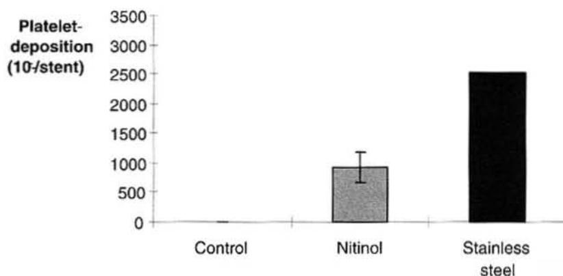
Figure 4 <sup>111</sup>In-platelet deposition on Nitinol stents, SS stents, and Silastic tubes (control) after 15 minutes of perfusion (\**p* < 0.001 vs. control).
