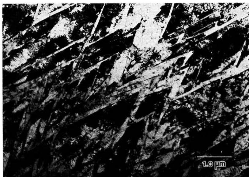
Fig. 1. Bright field image of twinned microstructure from a  $\text{Ti}_{50}\text{Ni}_{47}\text{Fe}_3$  alloy thermally cycled under a stress of 400 MPa.
