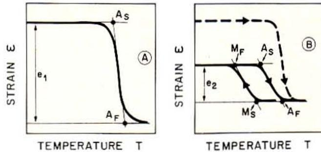
Figure 2. Illustration of a) the one-way shape-memory effect, and b) the two-way shape-memory effect. Note in b, that the  $A_S$  and  $A_F$  temperatures during initial heating are higher than those measured once full reversibility is achieved.
