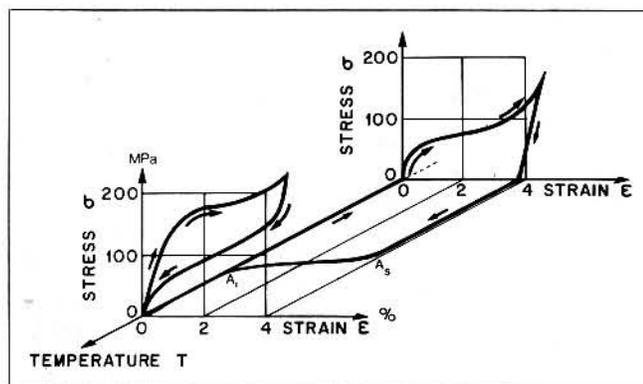
Figure 1. Tensile stress-strain-temperature map for NiTi shape-memory alloy.
