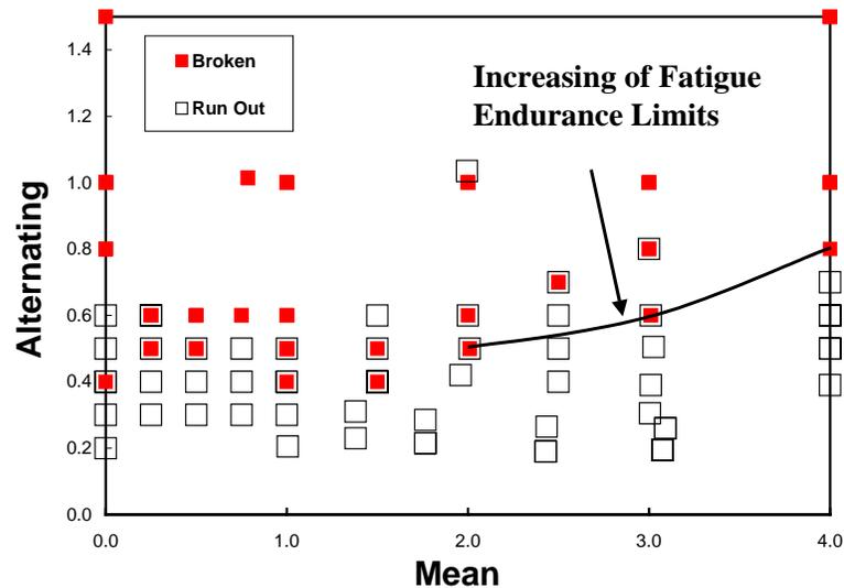
Fig. 1: Fatigue testing results on diamond shaped specimens.
