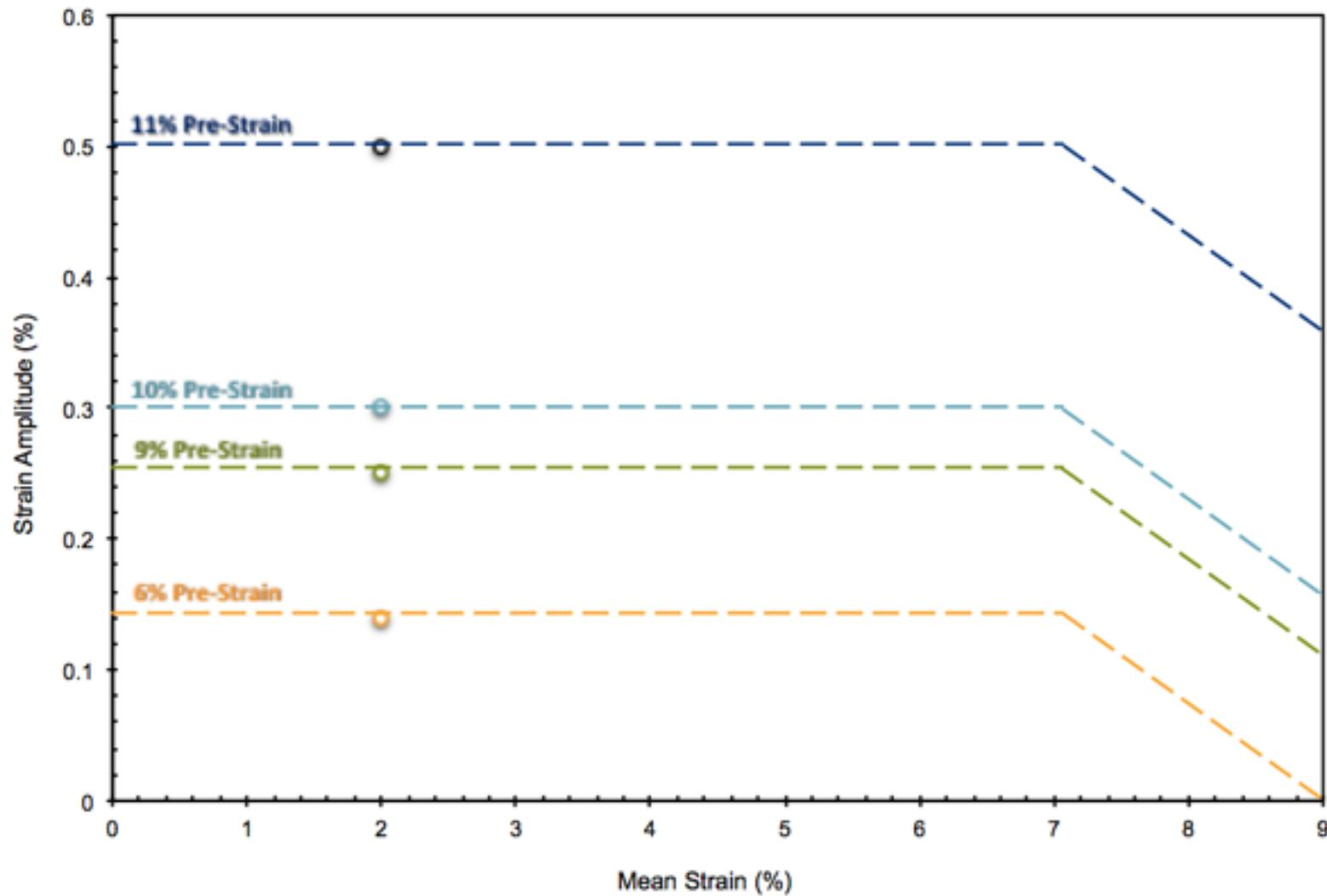
There are indications that increasing prestrain increases the fatigue safety threshold. Prestrain is potentially a third variable to consider when defining fatigue safety criteria, and when analyzing simulation results.
